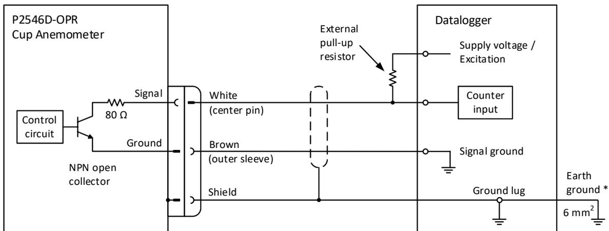
\* Connect the datalogger's ground lug to earth ground.
