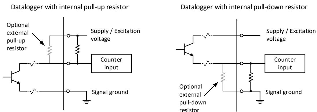
**Figure 2:** P2546D-OPR connection using an internal pull-up (left) or pull-down (right) resistor.
