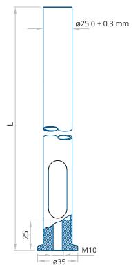
Mounting tube for power performance measurement
