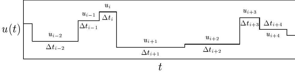
Figure 6. The sample-and-hold technique. We note that in this illustration, where the fluctuations are wildly exaggerated, that smaller values of  $u_i$  corresponds, as (56) shows, to larger values of  $\Delta t_i$ .
