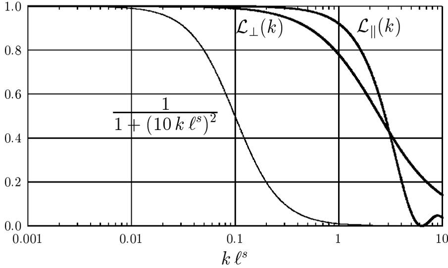
Figure 4. The two sonic transfer functions  $\mathcal{L}_{\parallel}(k)$  and  $\mathcal{L}_{\perp}(k)$  (thick line) as functions of  $k\ell^s = \omega\ell^s/U$  and a first-order filter (25) with  $\ell_o = 10 \times \ell^s$  (thin line).
