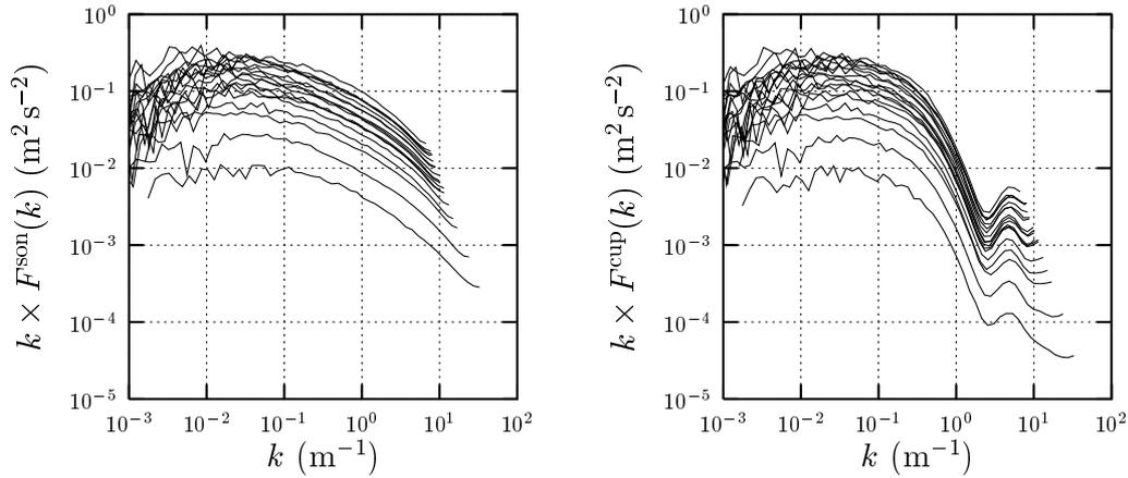
Figure 10. The spectra from the 18 periods as functions of the wave number  $k = \omega/U$ . There is a very close correspondence between the individual spectra from the sonic (left) and the cup (right).
